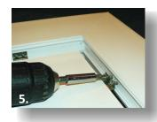
Fix each clip into the profile. It is not necessary for the screws to be driven right home.
